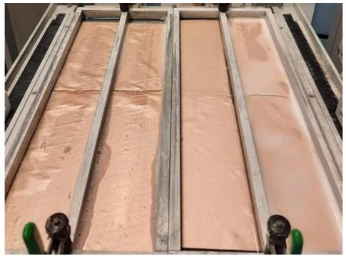
Figure 5. Test 1. Membrane with additive on the left and basic membrane on the right. Test time 1400 brushes. In the basic membrane, text begins to appear and the surface is broken at the embossed letters on the brushing path. Still no visible changes in the membrane with additive.
