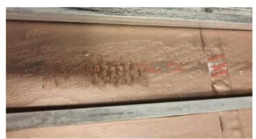
Figure 14. 200 brushes. In the part brushed with additional weights, detached coating appears precipitated on the surface.
