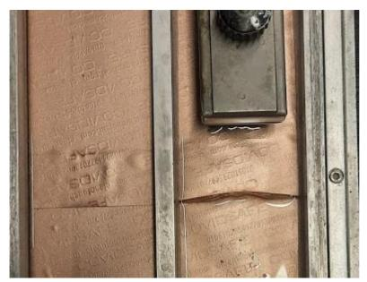
Figure 4. Test 1. Basic membrane at the seam after 600 brushes.
