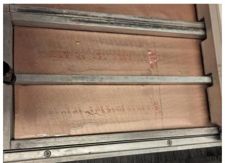
Figure 8. Test 2, additional weights on the basic membrane brushes. Basic membrane 600 brushes. In the basic membrane, the surface is broken at the embossed letters on the brushing path. The white base is exposed at the junction of the tape, which is raised from the rest of the membrane.
