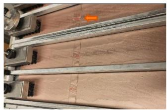
Figure 13. 133 brushes. In the basic brushing, text appears on the embossed part. With additional weights (top groove), the coating has punctured on the embossed part and the base has become visible.
