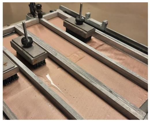
Figure 3. Test 1. Membrane with additive on the left and basic membrane on the right. Test time 600 brushes. In the basic membrane, red text appears at the seam. No visible changes in the membrane with additive.
