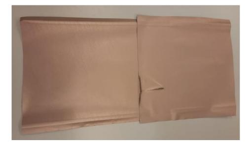
Figure 11. Test 2. Membrane with additive 4000 brushes. No visible changes on the membrane surface.
