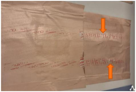
Figure 9. Test 2, additional weights on the basic membrane brushes. Basic membrane 2000 brushes. In the basic membrane, the surface is broken at the embossed letters on the brushing path. On the right side, the white base for a distance of approx. 10 cm is also exposed on the brushing path.
