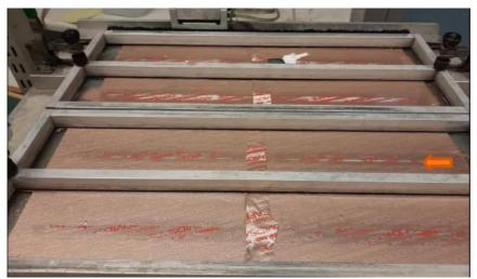
Figure 17. 1333 brushes. Coating punctured and white base visible in basic brushing. In brushing with additional weights (2 top notches), the coating is widely punctured and the tape is torn at the taping point (top notch).
